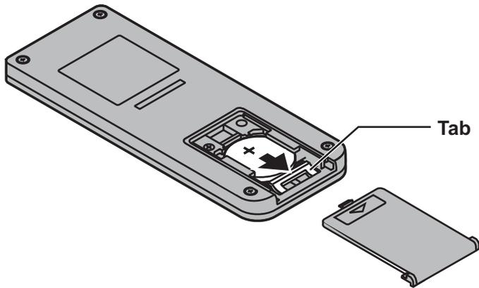
Pressing down on the tab, slide out the coin battery and remove.
