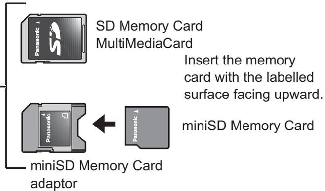
First insert the miniSD Memory Card into the card adaptor. Then insert the card adaptor into the memory card slot.
