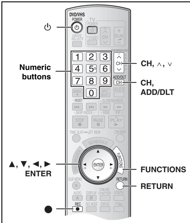
After plugging the unit into your household AC outlet and pressing [⏻, DVD/VHS POWER] to turn the unit on for the first time, the unit assists you to set the on-screen language, and automatically tunes in all the channels it can receive and sets the clock.
