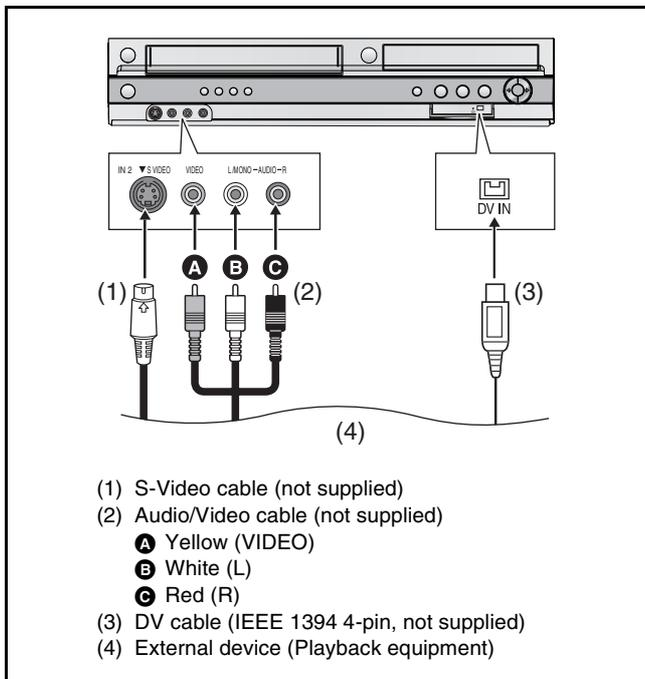
**Before connecting any cables, first make sure that the power for the unit and the external device are off. Then, after connecting cables, turn on both.**
