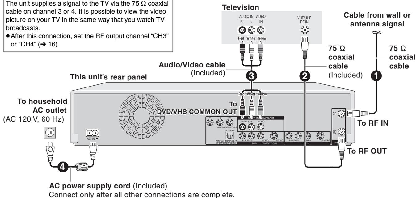
**B** Connection with a television and cable box or satellite receiver
