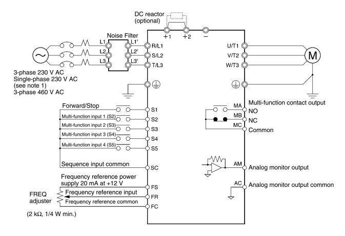
**Note** 1. Connect single-phase 230 V AC to terminals R/L1 and S/L2 of the 3G3JV-AB□.
