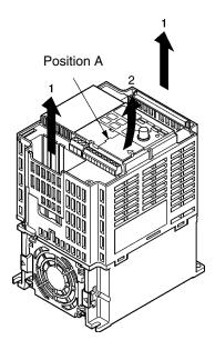
**Note** The front cover functions as a terminal cover. The Digital Operator cannot be removed.
