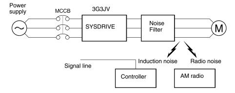
Induction Noise: Electromagnetic induction generates noise on the signal line, causing the con-
