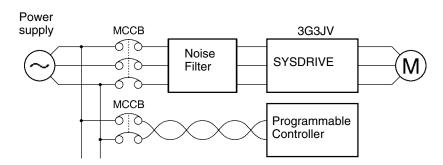
**Note** Use a Noise Filter designed for the Inverter. A general-purpose Noise Filter will be less effective and may not reduce noise.
