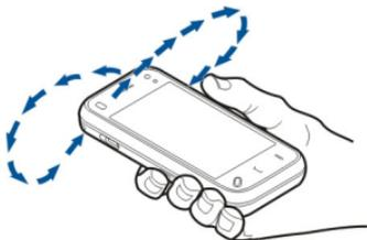
Rotate the device around all axes in a continuous movement until the calibration indicator changes its colour to green 🟢. If the indicator is yellow 🟡, the accuracy of the compass is low. If the indicator is red 🔴, the compass is not calibrated.
