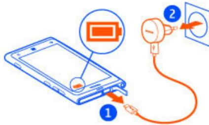
To avoid breaking the charger connector, be careful when connecting or disconnecting the charger cable.
