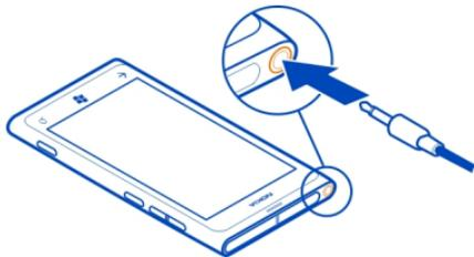
Do not connect products that create an output signal, as this may damage the device. Do not connect any voltage source to the audio connector. If you connect an external device or headset, other than those approved by Nokia for use with this device, to the audio connector, pay special attention to volume levels.
