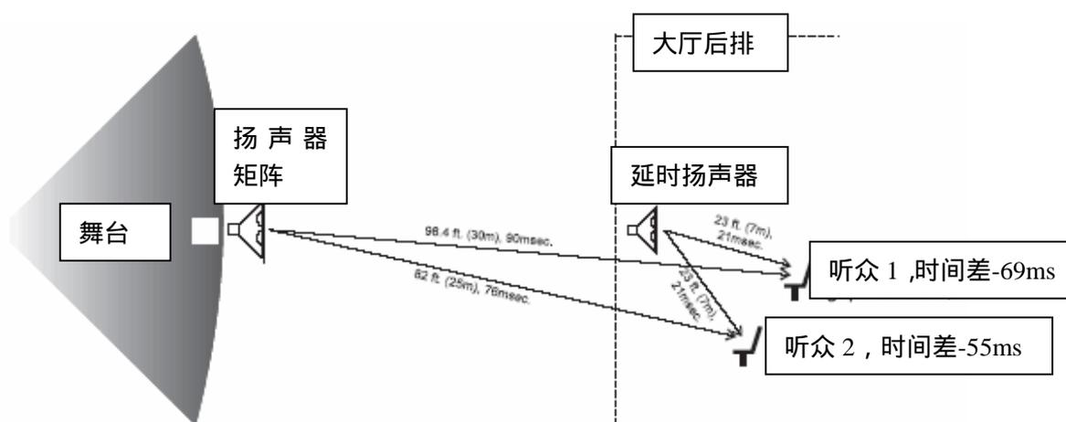
Delay Figure 5: Overhead view of under-balcony application.
