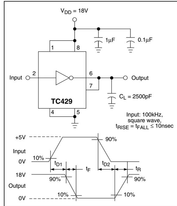
**FIGURE 3-2: SWITCHING SPEED**
