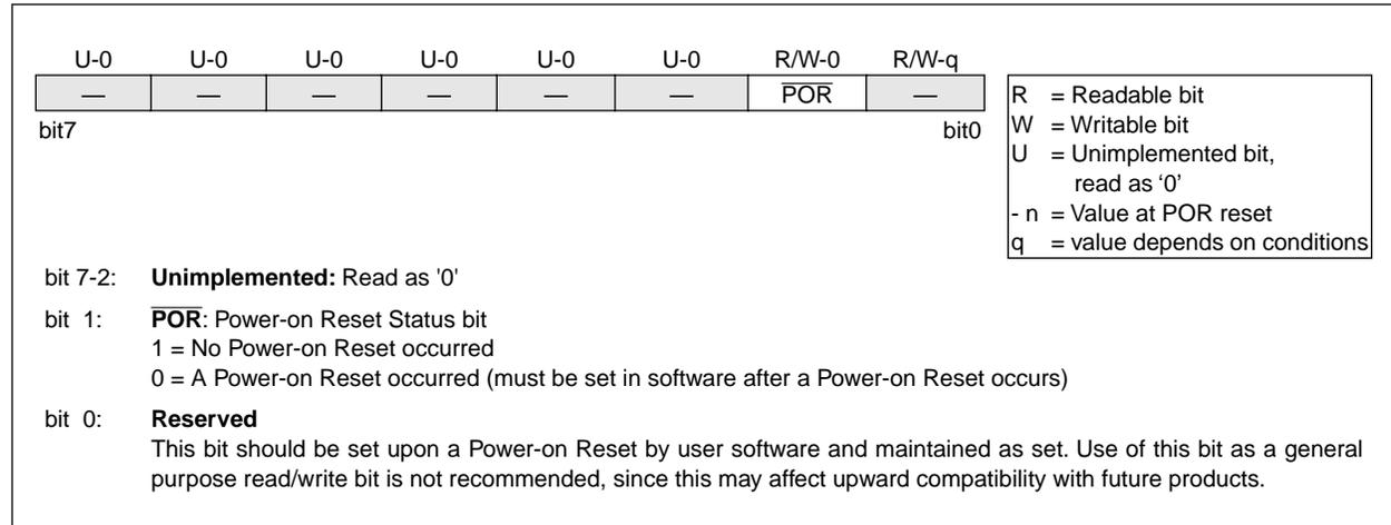
**FIGURE 4-23: PCON REGISTER FOR PIC16C62A/R62/63/R63/64A/R64/65A/R65/66/67 (ADDRESS 8Eh)**
