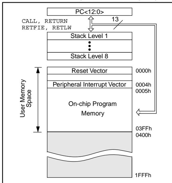
**FIGURE 4-2: PIC16C62/62A/R62/64/64A/R64 PROGRAM MEMORY MAP AND STACK**
