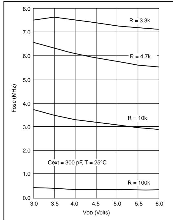
**FIGURE 17-3: TYPICAL RC OSCILLATOR FREQUENCY vs. VDD**
