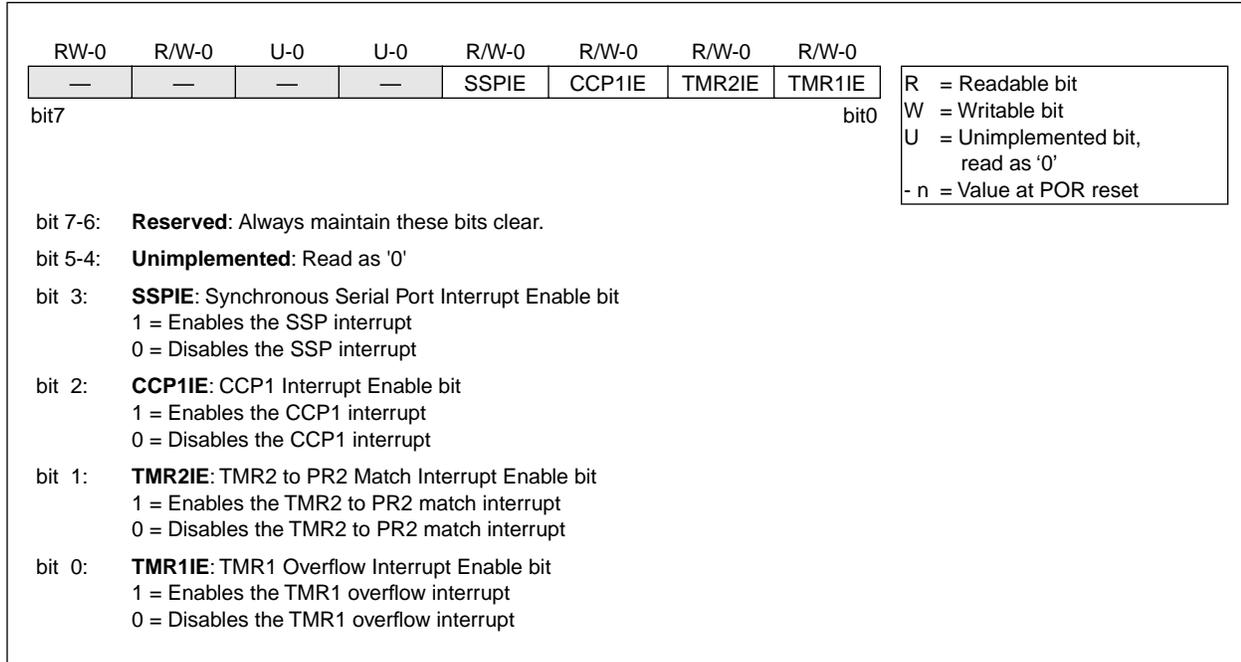
**FIGURE 4-13: PIE1 REGISTER FOR PIC16C63/R63/66 (ADDRESS 8Ch)**
