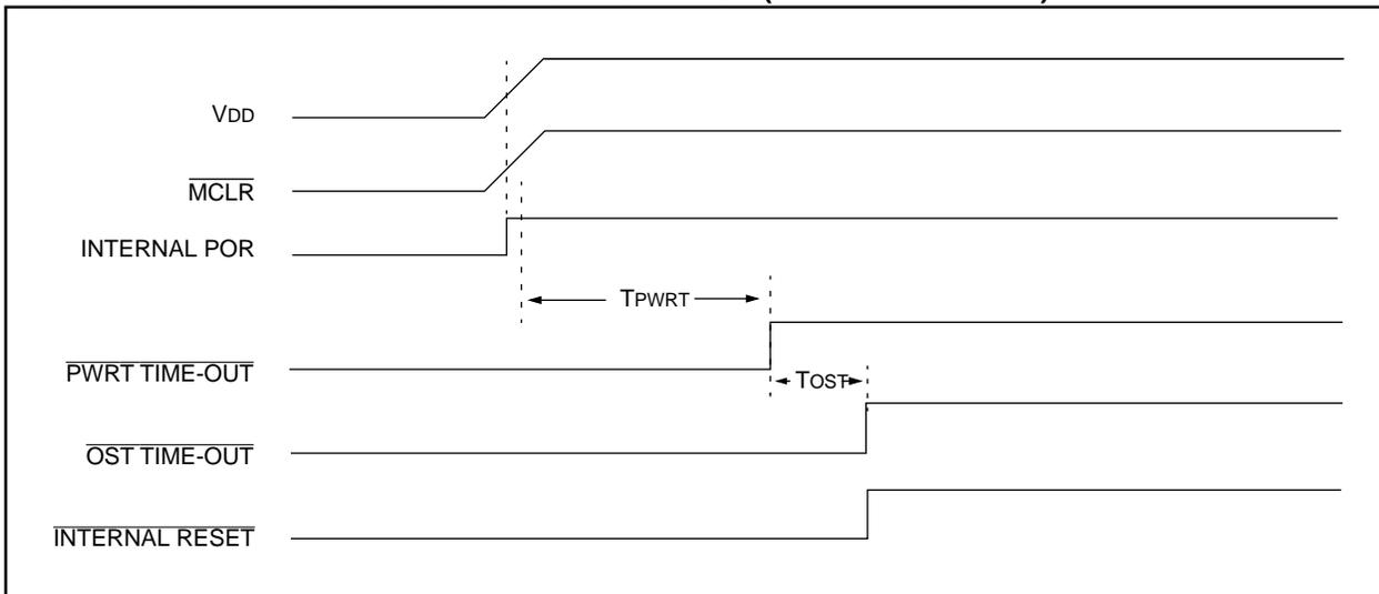
**FIGURE 13-14: EXTERNAL POWER-ON RESET CIRCUIT (FOR SLOW VDD POWER-UP)**
