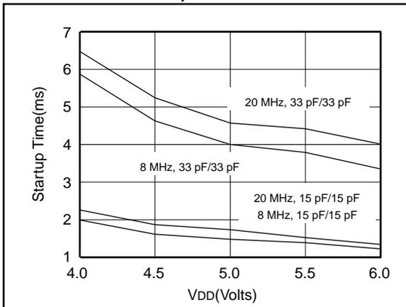
**FIGURE 24-24: TYPICAL XTAL STARTUP TIME vs. V<sub>DD</sub> (XT MODE, 25°C)**
