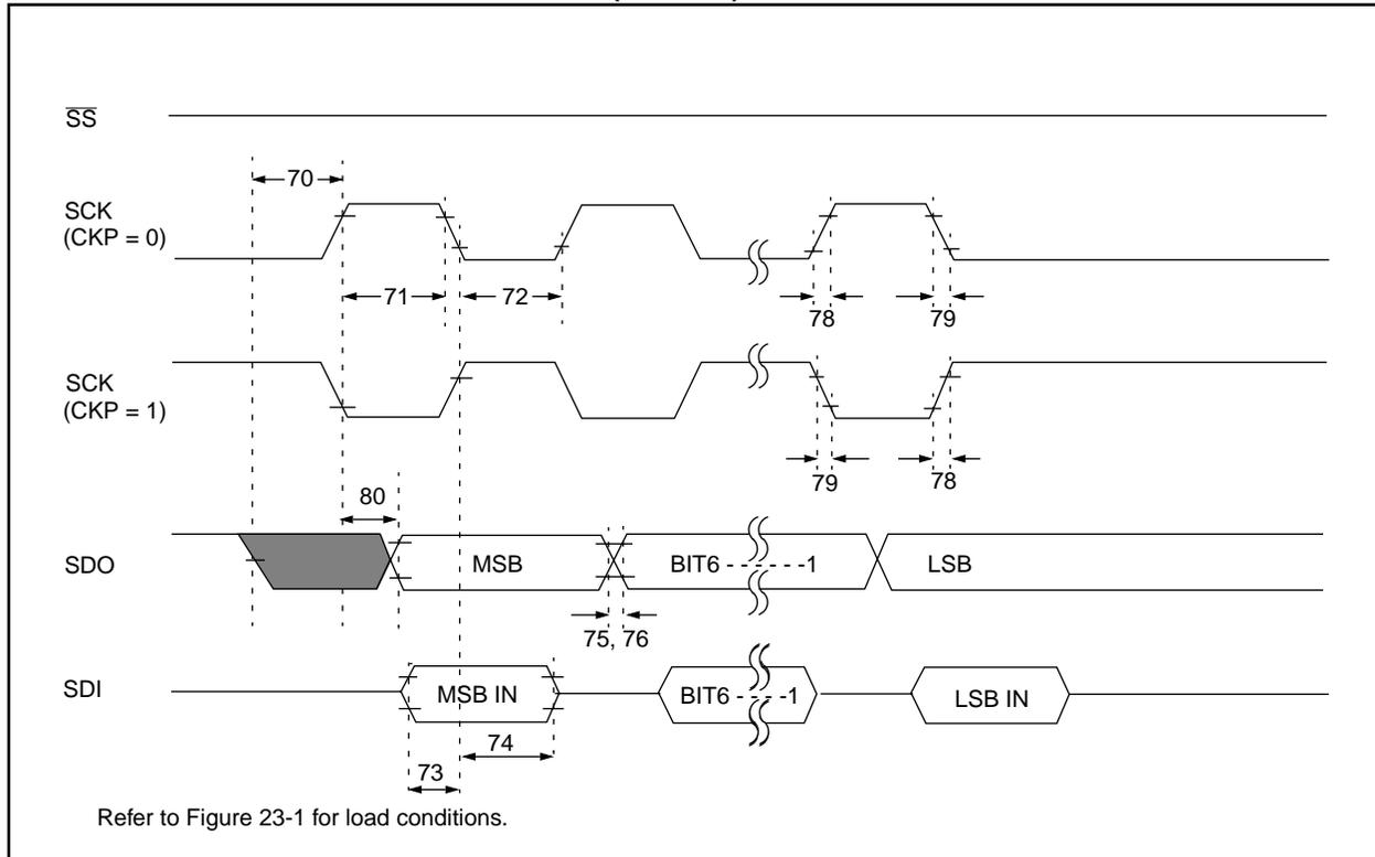
**FIGURE 23-10: SPI MASTER MODE TIMING (CKE = 1)**
