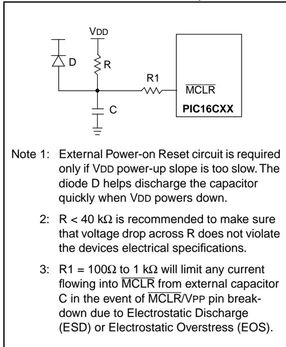
**FIGURE 13-15: EXTERNAL BROWN-OUT PROTECTION CIRCUIT 1**
