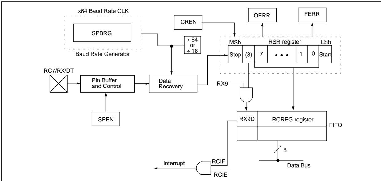
**FIGURE 12-11: ASYNCHRONOUS RECEPTION**
