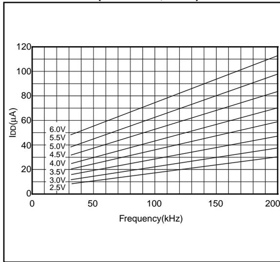
**FIGURE 24-27: TYPICAL  $I_{DD}$  vs. FREQUENCY (XT MODE, 25°C)**
