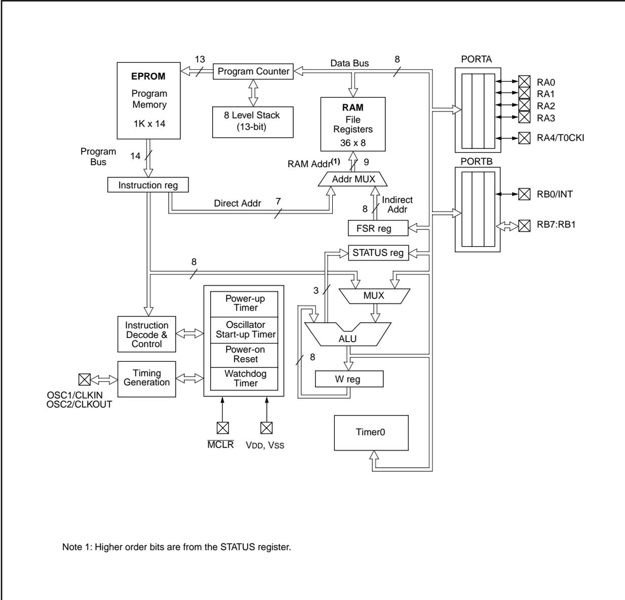
**FIGURE 3-2: PIC16C62/62A/R62/64/64A/R64 BLOCK DIAGRAM**
