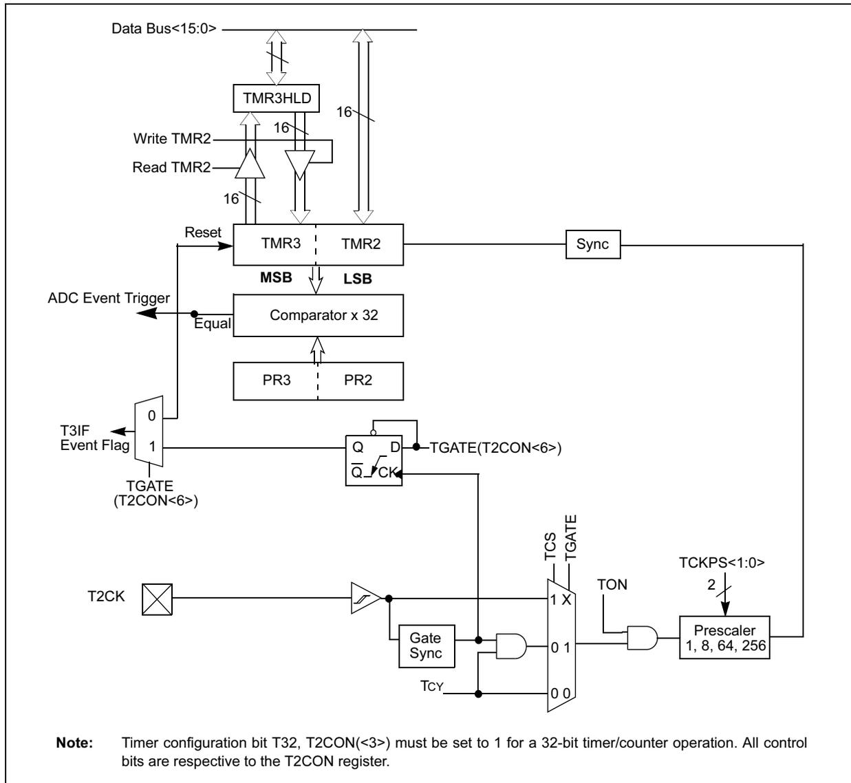
**FIGURE 10-2: 16-BIT TIMER2 BLOCK DIAGRAM**
