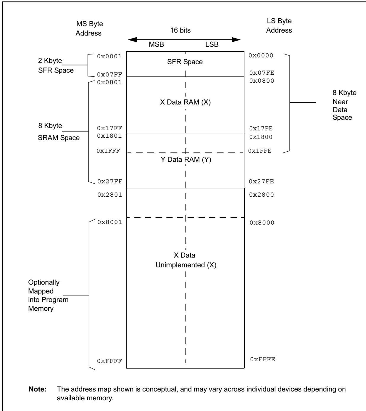
**FIGURE 3-9: DATA SPACE FOR MCU AND DSP (MAC CLASS) INSTRUCTIONS EXAMPLE**
