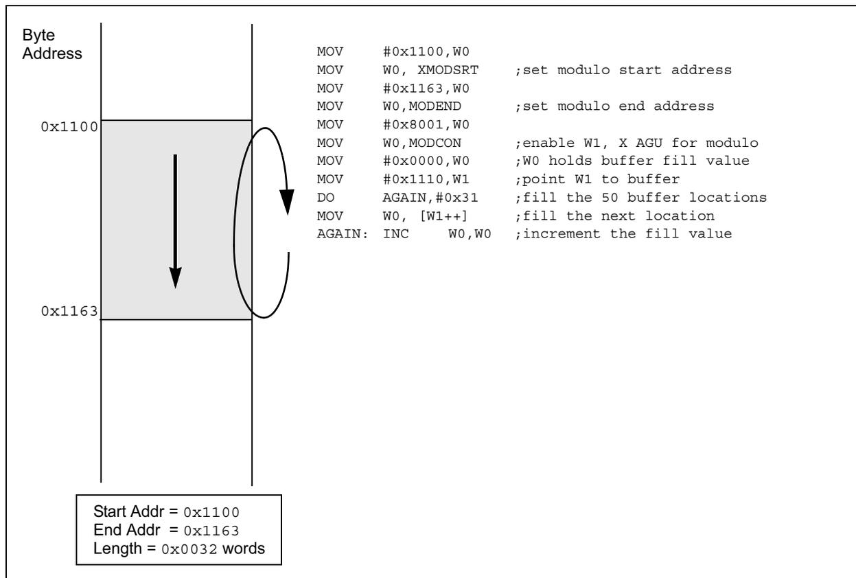
**FIGURE 4-2: DECREMENTING BUFFER MODULO ADDRESSING OPERATION EXAMPLE**
