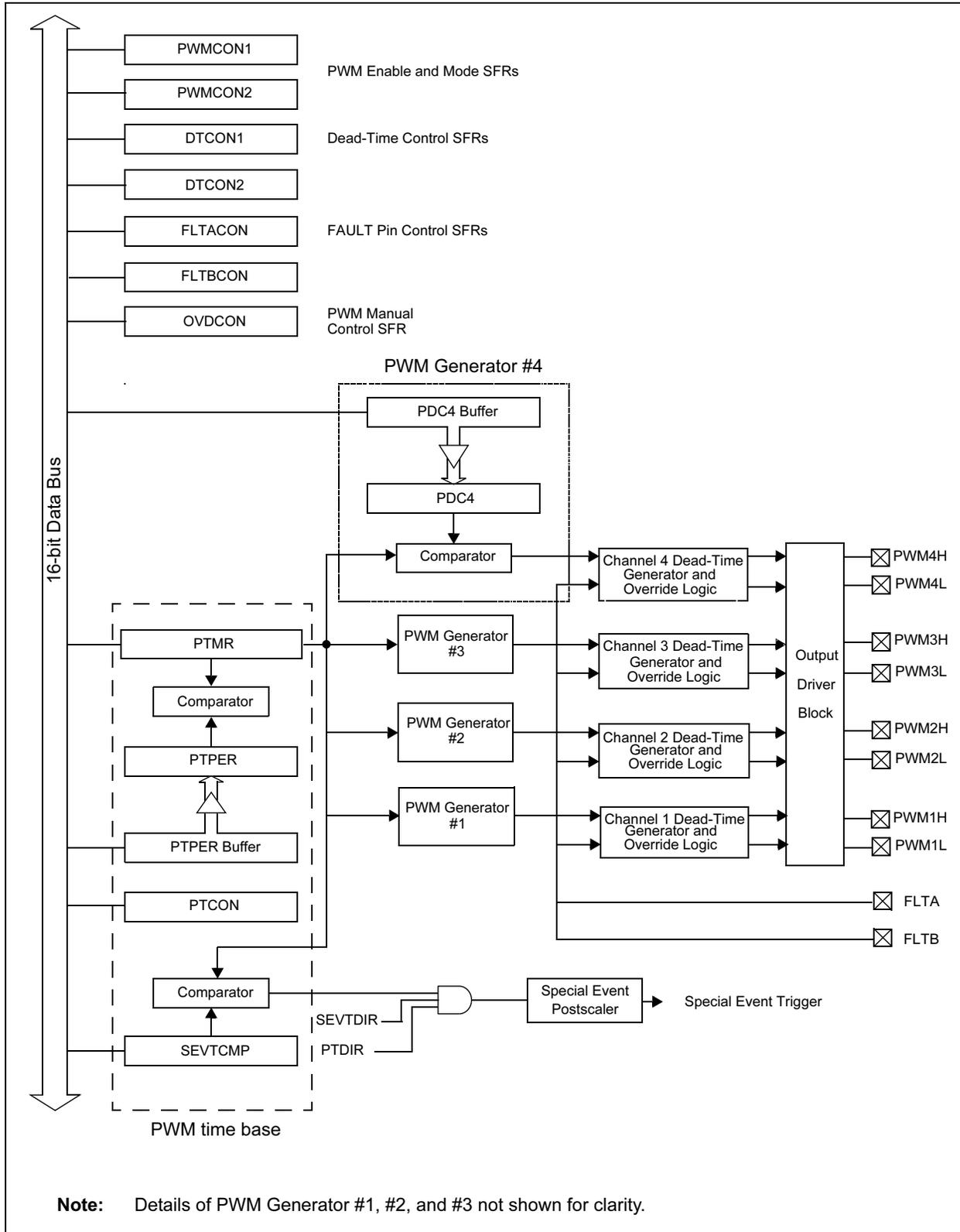
**FIGURE 15-2: 6-OUTPUT PWM BLOCK DIAGRAM**
