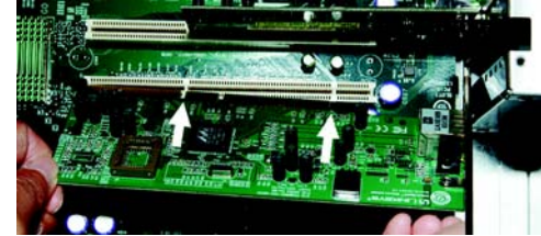
Figure 3-1: Insert the Adapter into the PCI Slot
