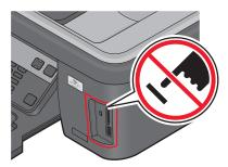
**Warning—Potential Damage:** Do not touch the USB cable, any network adapter, any connector, the memory device, or the printer in the areas shown while actively printing, reading, or writing from the memory device. A loss of data can occur.
