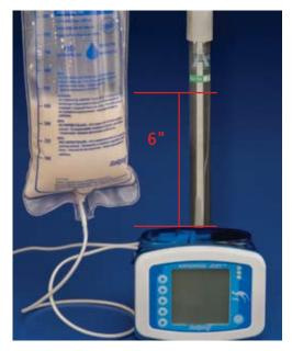
In order to achieve proper accuracy the initial fluid line in the feeding set container must be 6 inches above the top of the feeding pump when initiating the feeding cycle.
