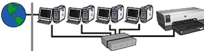
In this example, the network devices are connected to a [hub](#). A Macintosh OSX computer on the network acts as the [gateway](#) between the network and the Internet. The gateway
