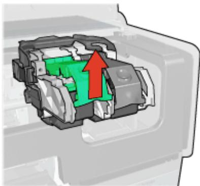
5. Slide the print cartridge out of the print cartridge cradle.
