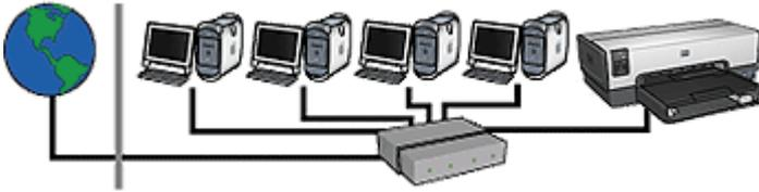
This example looks similar to the first example. However, in this example, the network devices are connected to a [hub](#), rather than a [router](#). The hub is directly connected to the Internet.
