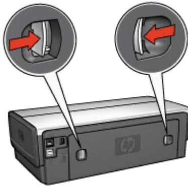
4. Remove any paper that is inside the printer by pulling it out from the back of the printer.
