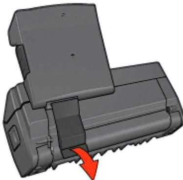
5. Tilt the Small Paper Tray forward and open the lower door of the accessory.
