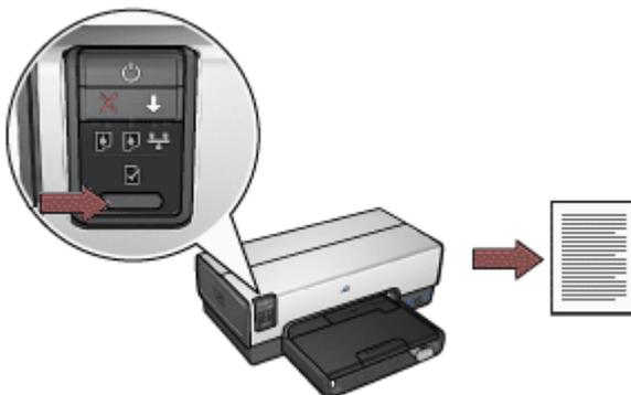
If the printer has just been connected to a network, wait a few minutes before printing the HP Report page to allow the printer to obtain valid settings.
