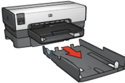
2. Slide the paper-width guide until the arrow is even with the correct setting.
