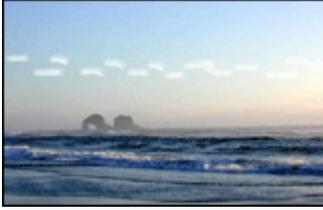
If streaks appear in a light portion of a photo, approximately 63 mm (2.5 inches) from one of the long edges of the photo, try the following solutions:
