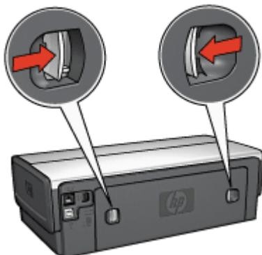
Do not discard the rear access door. In order to print, the accessory or the rear access door must be attached to the printer.
