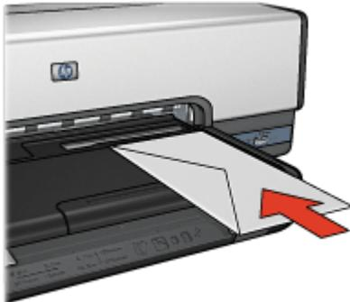
2. Push the envelope into the printer as far as it will go without bending.
