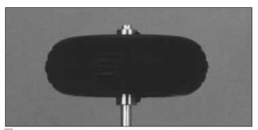
□ 1. Install the three **wheels** using the six **5/32**" **[4mm] wheel collars** and **set screws**. Grind or file a flat spot at the point of the set screw contact for each of the outer collars. This provides a better area for the set screw to "bite" and helps keep the wheels in place.
