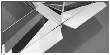
■ 4. Insert four hinges into the slots in the stabilizer. Press the elevators onto the hinges until the gap between the elevators and stabilizer is about 1/32" [.8mm]. Flex the elevators a little in one direction, but do not allow them to pull away from the stabilizer. Apply six drops of **thin CA** onto each
