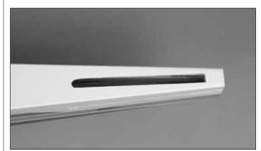
□ 2. Locate the slot for the vertical fin on the top of the fuselage and remove the covering.
