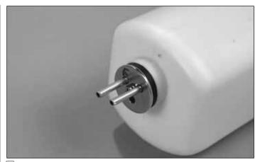
▲ 4. Push the stopper assembly into the tank and check the fit of the parts. The end of the bent tube should just touch the top of the tank. Rotate the tank around with the stopper facing up. The clunk should not touch the back of the tank. When the parts fit properly, tighten the screw on the stopper assembly. Mark the tube that is connected to the clunk. In the above photo, we marked the tube on the right side of the tank with an "F", for fuel.
