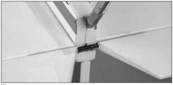
5. **Carefully** cut a slot in the tail post using a hobby knife for the lower rudder hinge.
