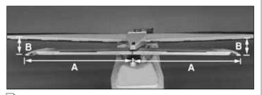
▲ 4. Insert the stabilizer into the stabilizer slot so it is centered in the fuselage (dimension A should be equal). Place the wing onto the fuselage and secure it in place with the wing hold-down bolts. View the plane from the rear and at a distance of a few feet. The stabilizer should be parallel to the wing (dimension B should be equal). If not, sand the stabilizer mounting base slightly to achieve the proper position of the stabilizer.
