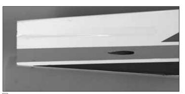
□ 1. Locate the pushrod exit slot under the covering on the tail section of the fuselage by lightly pressing with your fingers. The slot should be located 4" [102mm] from the rear the fuselage and 3/4" [19mm] from the bottom of the fuselage. Trim the covering to provide access to the pushrod exit.
