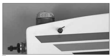
□ 1. Mark the position of the needle valve for your engine installation. Also, mark the fuselage for any cutouts you will need for the muffler, then remove the engine from the mount. Cut or drill the fuselage side to allow for ease of needle valve adjustments. Leave a space around the needle valve so that any vibrations will not affect the needle setting.
