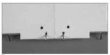
□ 3. Turn the wing over and remove the covering from the holes for the wing bolts. Using a 1/4" [6.4mm] drill bit, drill holes through the wing bolt plate for the wing bolts.
