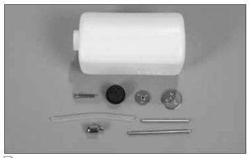
□ 1. Locate the parts for the fuel tank. You will need only one long and one short aluminum tube. Cut the silicone fuel tube to a length of 3-1/2" [89mm].
