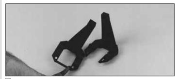
□ 1. Remove the center spreader from the **engine mount** halves. Trim any excess flashing with a hobby knife or file.
