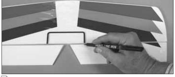
□ 1. Without glue, position the **elevator halves** on the **stabilizer**. Measure and mark a centerline onto the elevator joiner wire. Center the joiner between the two elevator halves. Mark the position where the joiner will enter the elevator halves.
