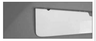
□ 6. Temporarily install the rudder to determine where to notch the rudder to allow clearance for the elevator joiner. Press the rudder gently to leave an impression of the joiner on the rudder. Remove the rudder and cut a notch that is 1/16" [1.6mm] above and below the impression. The notch should be cut 1/4" [6.4mm] deep.
