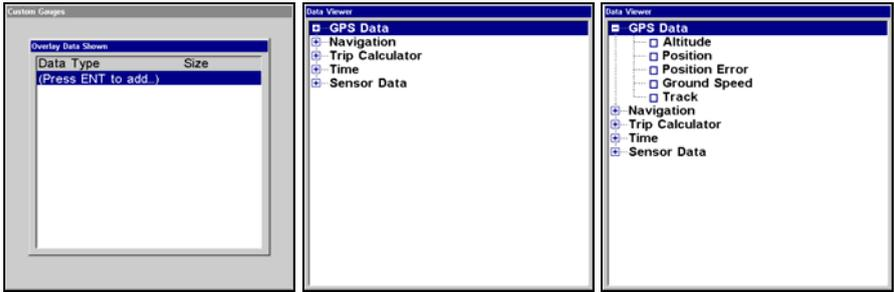
**Highlight PRESS ENT TO ADD... and press ENT in the Overlay Data Shown menu (far left) to open the Data Viewer menu (center) with five expandable data categories: GPS Data, Navigation, Trip Calculator, Time and Sensor Data. The right figure shows the subcategory list under the GPS Data category.**
