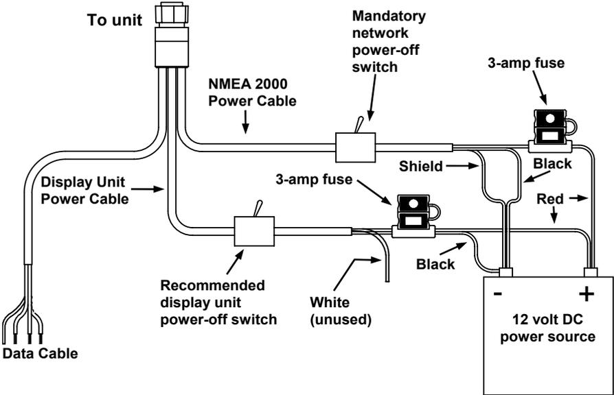
Use this method if you are powering the display unit and a GPS module or the display unit and a NMEA 2000 network. (Fuses may be different from those shown.).
