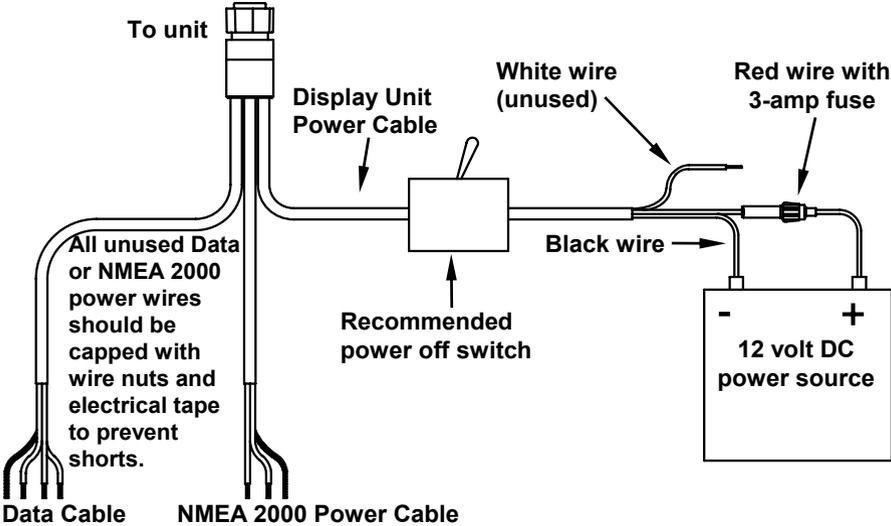
Use this method if you are *only* powering your display unit and are not powering a NMEA 2000 network or any NMEA 2000 accessory device, including a GPS module. (Fuse may be different from that shown.)
