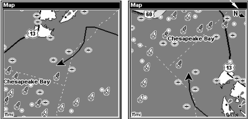
Map orientation at left is shown in north up and at right, track up.
