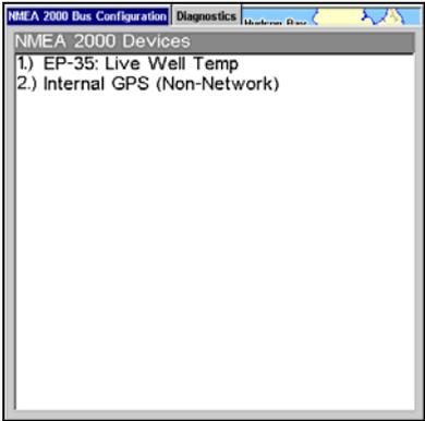
**If you do not have an EP-15 Fluid Level, EP-10 Fuel Flow or EP-20 Engine Interface on the network, the Bus Configuration menu will not display the Engine-Tank Configuration menu, Tank Select menu, Tank Size menu or Set Configuration button.**
