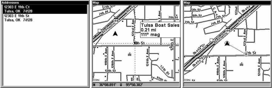
Address search result list, left. At center, Map Page showing location of the address on the map, highlighted by cursor. At right, after the address is located, you can navigate to it ("D" symbol for destination).
