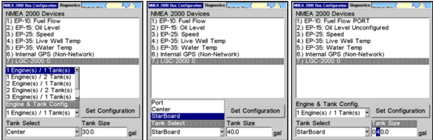
**1 Engine/1Tank highlighted on Engine and Tank Configuration menu (left). Starboard highlighted on Tank Select menu (center). Tank Size set to 40 gallons (right).**
