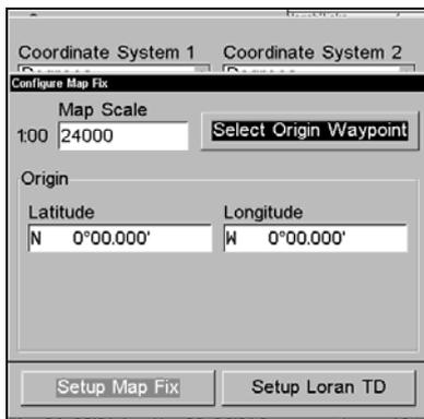
**Configure a map fix so the unit can find your position on a printed chart or topographical map.**
