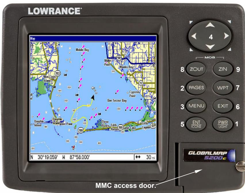
The GlobalMap 5200c GPS unit Map Page, keyboard and access door for the MMC slot.
