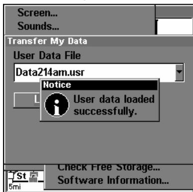
These figures show the menu sequence for loading a GPS Data File from an MMC into the unit's memory.
