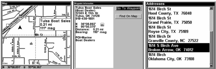
Left, Map Page showing location of the address on the map, highlighted by cursor. Center, this address is a business in the POI database, so you can display the POI information window, then navigate to it. At right, this address is not in the POI database, so the Waypoint key will not display any information for this address.
