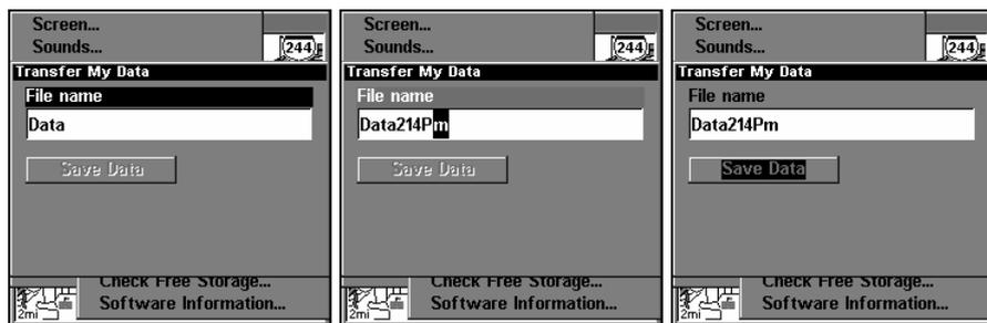
From left to right, these figures show the menu sequence for naming and saving a GPS Data File from the unit's memory to an MMC.
