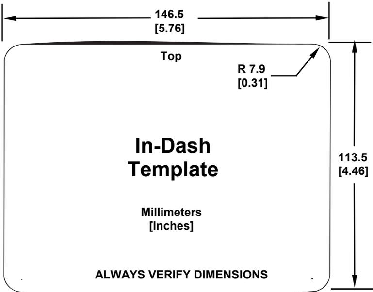
In-dash mounting template for the GlobalMap 5200c, showing dimensions. NOTE: The figure above is *not* printed to scale. A scaled template (FM-5 In-Dash Adapter Kit instructions) is available for free download from our web site, [www.lowrance.com](http://www.lowrance.com).
