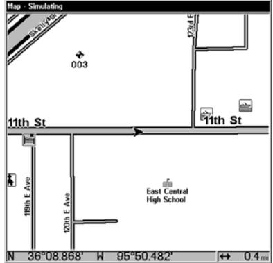
Sequence for setting a waypoint. Step 1: while traveling, *quickly* press **WPT twice** to call up Find Waypoint screen (seen in Step 2) and set a point. Step 3: a message says the waypoint has been saved. Step 4: vehicle continues on its way; number waypoint symbol is visible on map.
