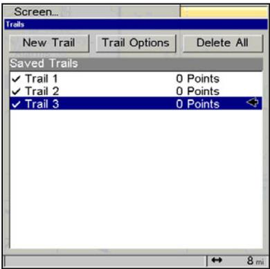
New trail, named "Trail 3" is created when Trail 2 is made inactive. Any new travel will be recorded in this trail, which is active and visible. Trails do not need to be visible in order to be active.
