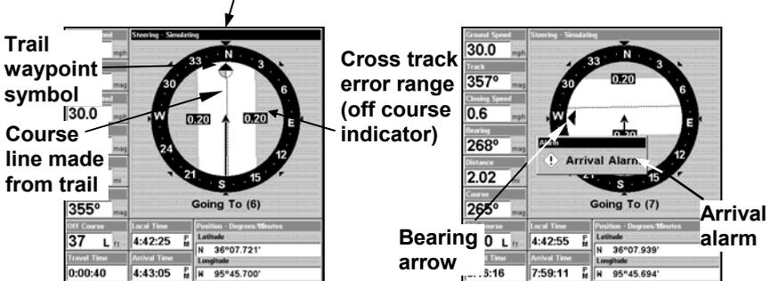
Navigate trail, navigation page (compass rose) views: at left, driver is northbound heading straight toward trail point 6; bearing arrow shows the trail point is due north (straight ahead.) At right, driver has reached trail point 6 and must turn west to follow the trail. Arrival alarm goes off and bearing arrow swings around to say turn left (west), toward the next waypoint, trail point 7. The unit now shows navigation information to point 7, which is 2.02 miles away.
