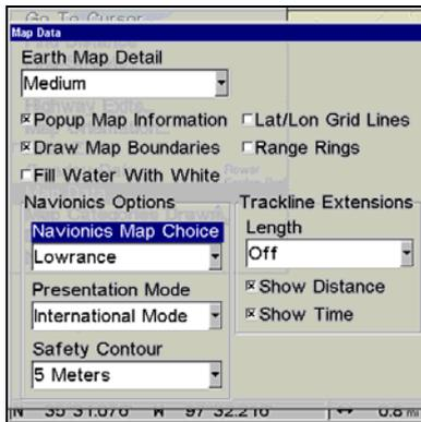
Navionics Map Choice highlighted. Press Ent to select the desired Navionics map from the Map Choice drop down box.
