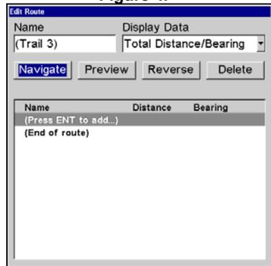
Navigate a trail menu sequence: Fig. 1, My Trails command. Fig. 2, Trails Menu. Fig. 3, Edit Trail Menu. Fig. 4, Edit Route Menu for Trail 3. A trail is always converted to a "route" when you navigate the trail.
