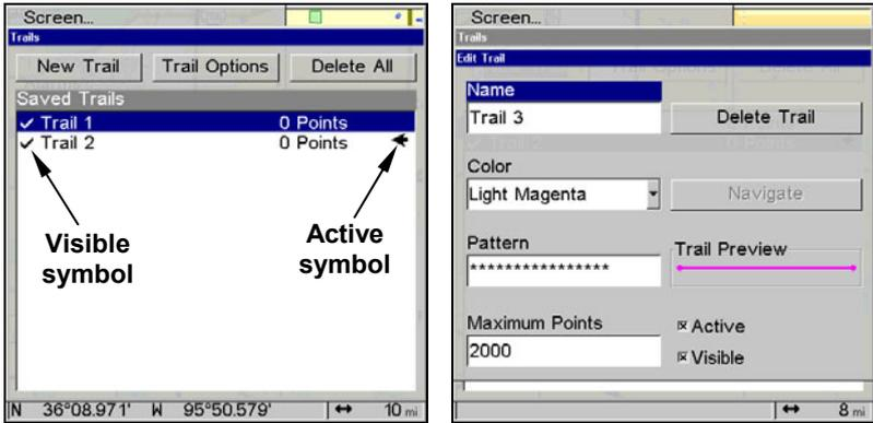
Sequence for saving a trail and beginning a new one, after My Trails command is selected. The Trails Menu, at left. The arrow to the right of Trail 2 indicates the trail is "active" and the check to the left indicates the trail is visible on the map display. The right figure shows the Edit Trail menu, with the Active and Visible commands selected.
