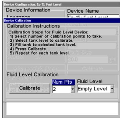
**Calibrate is highlighted on the device configuration menu (left). Calibration menu (right) with calibration instructions listed at the top.**
