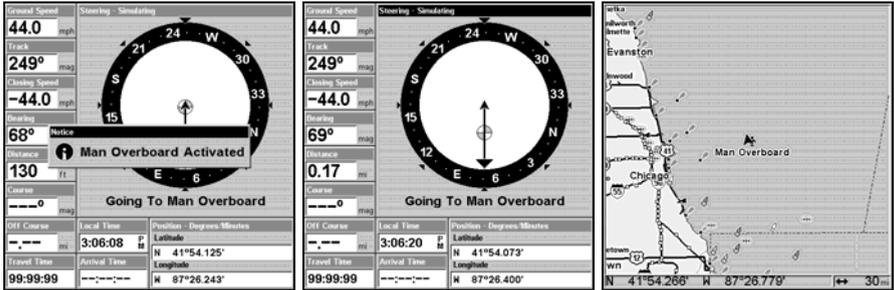
Navigating to Man Overboard: Man Overboard Activated message, left, Navigation Page, center, Map Page, right. The MOB is to the starboard of the vessel; the GPS shows which direction to steer for the rescue.
