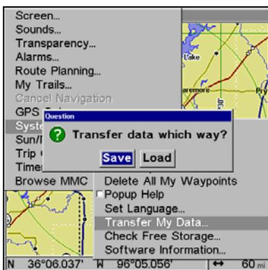
The **Transfer My Data** submenu asks if you want to save data to the MMC or load data from the MMC into the unit's memory.
