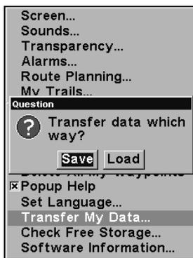
The **Transfer My Data** submenu asks if you want to save data to the MMC or load data from the MMC into the unit's memory.
