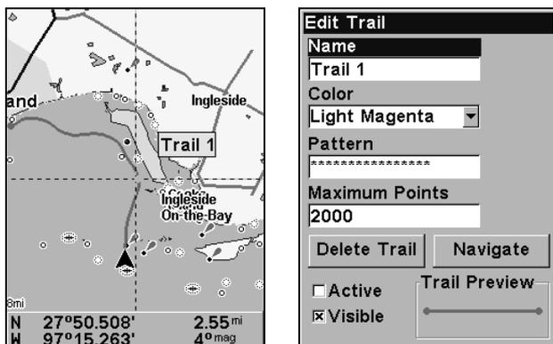
At left, trail selected with map cursor. The box at the bottom of the screen shows distance and bearing from current position to the selected point on the trail. At right, the Edit Trail menu.
