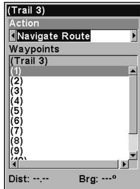
Navigate a trail menu sequence: Fig. 1, My Trails command. Fig. 2, Trails Menu. Fig. 3, Edit Trail Menu. Fig. 4, Edit Route Menu with Navigate Route command highlighted for Trail 1. A trail is always converted to a "route" when you navigate the trail.
