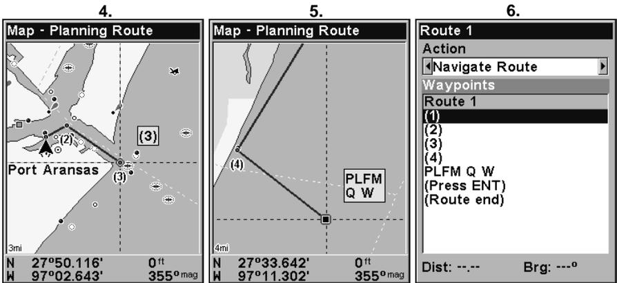
Route creation sequence, continued: Fig. 4. Point (3) set at channel mouth. Fig. 5. Waypoint (4) set further south along the beach, at a recognizable landmark (Bob Hall Pier). Waypoint PLFM Q W ends the route at an oil platform some distance from the shore. Fig. 6. Press EXIT to save the route and you return to this screen.
