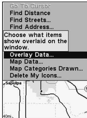
System Setup Menu, left, with Pop-up Help command highlighted. At right, this example shows the Pop-up Help message for the Overlay Data command, located on the Map Page menu.
