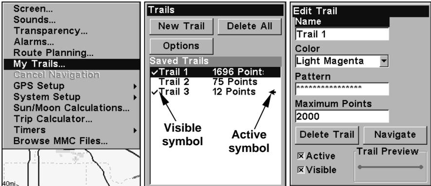
Sequence for saving a trail and beginning a new one. At left, My Trails command. Center, the Trails Menu. The arrow to the right of Trail 3 indicates the trail is "active," and the check to the left indicates the trail is visible on the map display. The right figure shows the Edit Trail menu, with the Name command selected.
