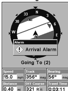
Navigating along a route: Fig. 1 shows the Navigation Page at the start of a route, heading straight for the first waypoint (Wpt 1). In Fig. 2, the traveler has arrived at Wpt 1; the arrival alarm has been triggered and the bearing arrow on the compass rose has turned to point toward Wpt 2, off to the northeast.
