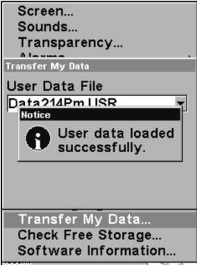
These figures show the menu sequence for loading a GPS Data File from an MMC into the unit's memory.
