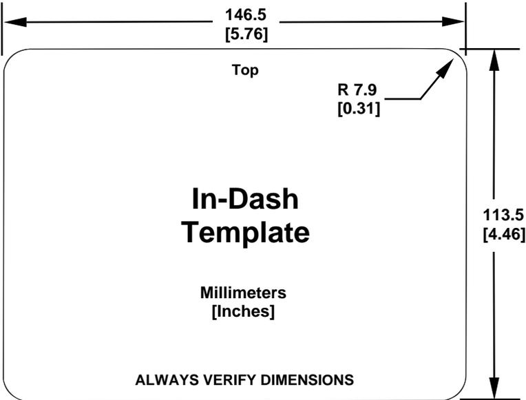
In-dash mounting template for GlobalMap 3300C GPS unit, showing dimensions. NOTE: The figure above is *not* printed to scale. A scaled template (FM-5 In-Dash Adapter Kit instructions) is available for free download from our web site, [www.lowrance.com](http://www.lowrance.com).
