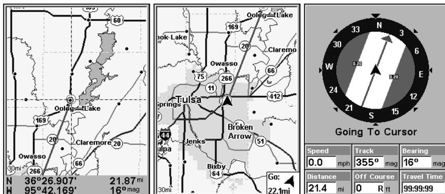
The 30-mile zoom figure at left clearly shows the red course line connecting your current position to your destination. The 30-mile zoom, center, shows both current position and direction to destination on screen. The Navigation Page, right, will also show navigation information.
