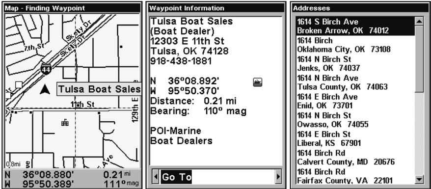
Left, Map Page showing location of the address on the map, highlighted by cursor. Center, this address is a business in the POI database, so you can display the POI information window, then navigate to it. At right, this address is not in the POI database, so the Waypoint key will not display any information for this address.
