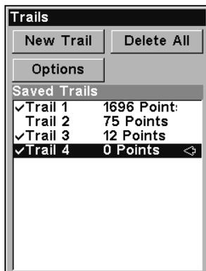
New trail, named "Trail 4," is created when Trail 3 is made inactive. Any new travel will be recorded in this trail, which is active and visible. Trails do not need to be visible in order to be active.
