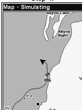
Sequence for setting a waypoint. Step 1: while traveling, *quickly* press **WPT** twice to call up Find Waypoint screen (seen in Step 2) and set a point. Step 3: a message says the waypoint has been saved. Step 4: vehicle continues on its way; number waypoint symbol is visible on map.
