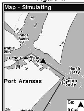
In Fig. 3 the traveler has turned northeast on his new course and is heading straight for Wpt 2, which is 0.27 miles away. Fig. 4 shows route navigation on the Map Page. In this figure, the traveler has reached Wpt 2 and is starting on the leg between Wpts 2 and 3.
