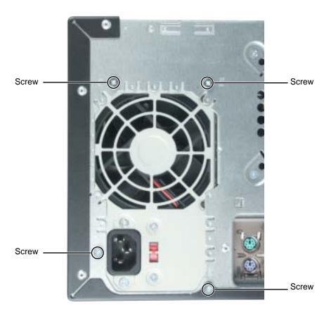
**5** Slide the power supply up and away from the power supply brackets.
