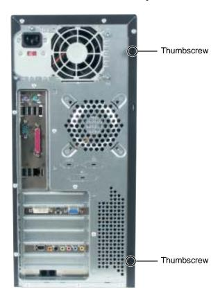
**5** Slide the side panel toward the back of the computer, then pull the panel away from the computer.
