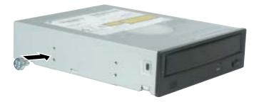
**10** Slide the new drive into the drive bay. Push firmly until the drive release latch locks the drive into place.
