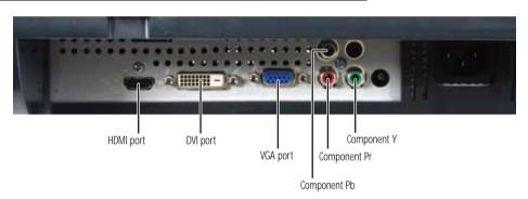
3 Make sure that your computer is turned off, then connect the other end of the video cable to the matching video port on the back of your computer.
