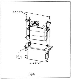
3. The use of a servo tray is extremely convenient when installing the servos. The method of installation is illustrated in the figure 6. (Insert each connector fully.) Don't forget to confirm that the motion of the servo horns and rods matches the direction of operation of the transmitter sticks. Use the reversible servo
