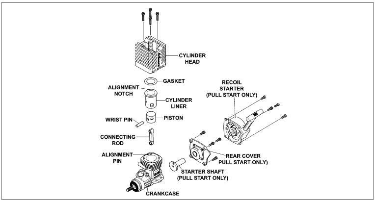
How to install your new DuraTrax piston/cylinder assembly into your O.S.® Max® .12 Series R/C engine:
