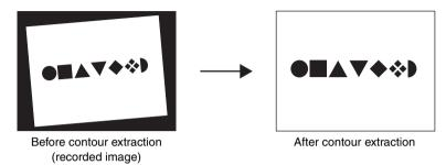
Contour extraction is performed automatically when Trapezoid Correction is turned on. You can use any one of the operations below to toggle Trapezoid Correction on and off.
