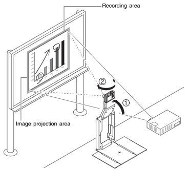
Point the camera at the whiteboard so it is at an angle that is within the allowable range.
