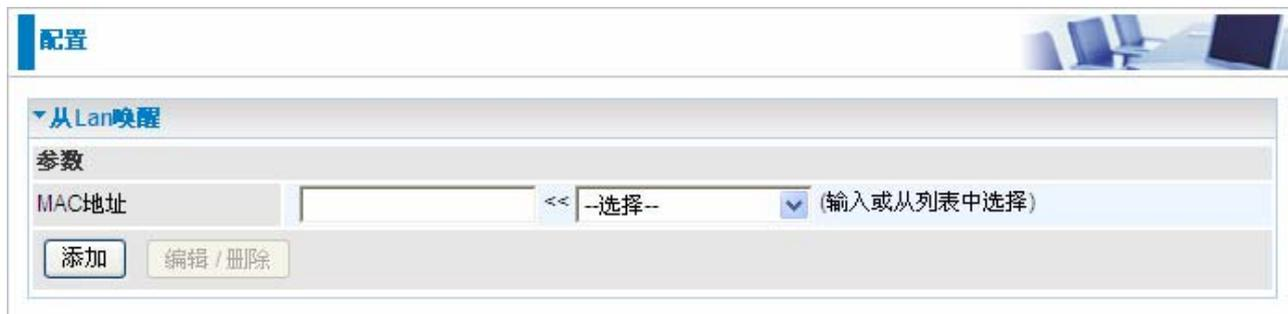
The screenshot shows a configuration window titled "配置" (Configuration). Under the "从 Lan 唤醒" (Wake Up from LAN) section, there is a "参数" (Parameters) area. It contains a "MAC地址" (MAC Address) field with a text input box, a dropdown menu showing "--选择--" (Select), and a note "(输入或从列表中选择)" (Enter or select from list). Below the input field are two buttons: "添加" (Add) and "编辑 / 删除" (Edit / Delete).
