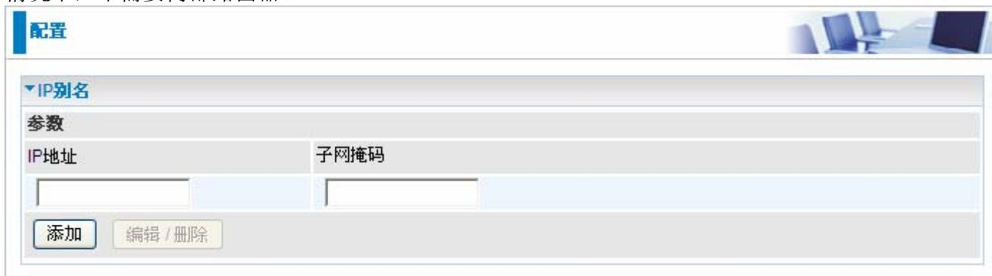
The screenshot shows the '配置' (Configuration) menu with the 'IP别名' (IP Alias) sub-menu expanded. Under '参数' (Parameters), there are two input fields: 'IP地址' (IP Address) and '子网掩码' (Subnet Mask). At the bottom, there are two buttons: '添加' (Add) and '编辑/删除' (Edit/Delete).
