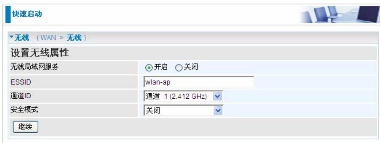
The screenshot shows the '快速启动' (Quick Start) configuration page for wireless settings. The breadcrumb is 'WAN > 无线'. The main heading is '设置无线属性' (Set Wireless Properties). The '无线局域网服务' (Wireless LAN Service) is set to '开启' (On). The 'ESSID' is set to 'wlan-ap'. The '通道ID' (Channel ID) is set to '通道 1 (2.412 GHz)'. The '安全模式' (Security Mode) is set to '关闭'. There is a '继续' (Continue) button.
