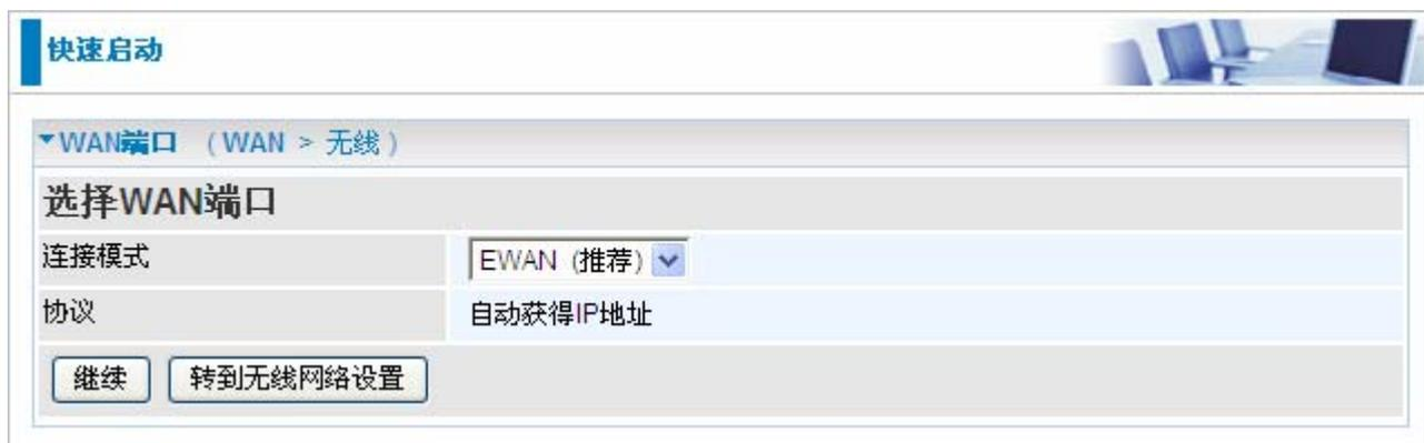
The screenshot shows the '快速启动' (Quick Start) configuration page. The breadcrumb is 'WAN > 无线'. The main heading is '选择WAN端口' (Select WAN Port). The '连接模式' (Connection Mode) is set to 'EWAN (推荐)' (EWAN (Recommended)). The '协议' (Protocol) is set to '自动获得IP地址' (Obtain IP address automatically). There are two buttons: '继续' (Continue) and '转到无线网络设置' (Go to Wireless Network Settings).
