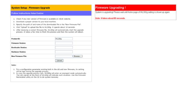
This page reports the Flash Code (Firmware) version installed in the ASUS 802.11g AP. Periodically, a new Flash Code is available for the ASUS 802.11g APs on ASUS's Web site. You can update the ASUS 802.11g AP's Flash Code using the Firmware Upgrade page under the Advanced Setup menu of the Web Manager. If you are experiencing a problem with your ASUS WLAN equipment, a Technical Support representative may ask you to give your device's Flash Code (Firmware) version.
