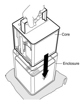
With a flat hand, press down on the latch until it locks into place. Firmly press the core to ensure it is fully secured within the enclosure.
