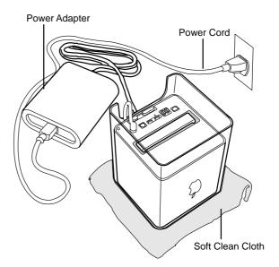
**Important:** To avoid electrostatic discharge, always ground yourself by touching the port access covers before you touch any parts or install any components inside the computer. To avoid static electricity building back up in your body, do not walk around the room until you have completed the installation and closed the computer.
