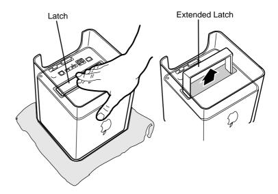
Allow the latch to extend completely.
