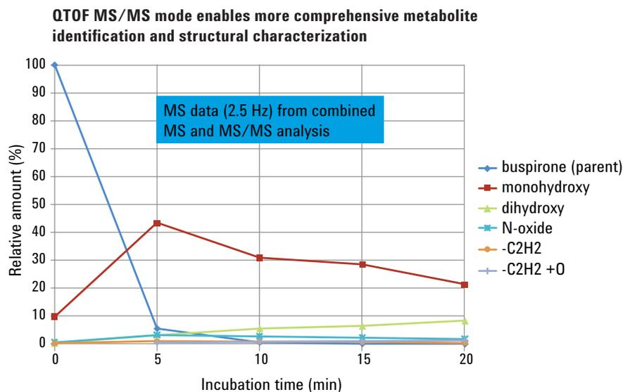
Figure 5. Metabolic stability and metabolic profiling from the same experiment (combined MS and MS/MS, MS at 2.5 Hz acquisition rate) with the Agilent 6540 QTOF. Graph assumes all response factors were the same as for the parent buspirone.
