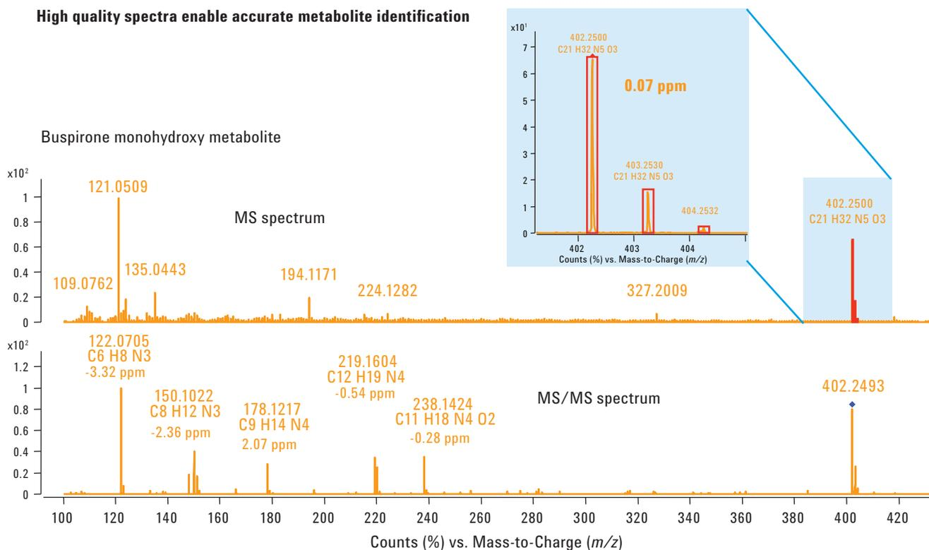
*Figure 6. The molecular formula generation algorithm identified the metabolites by taking advantage of both the excellent match of the precursor isotope pattern and the mass agreement for precursor and product ions.*
