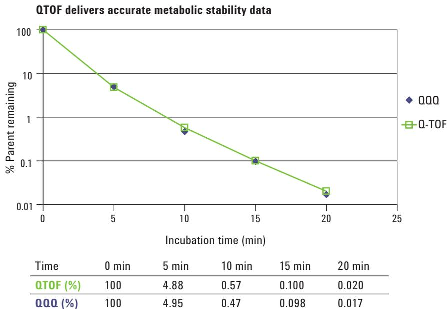
*Figure 1. The 6540 QTOF gave metabolic stability results for buspirone that were in good agreement with those obtained using the 6460 Triple Quadrupole system. Results are plotted using a semi-log scale (log %Parent remaining) to provide a linear relationship to incubation time.*
