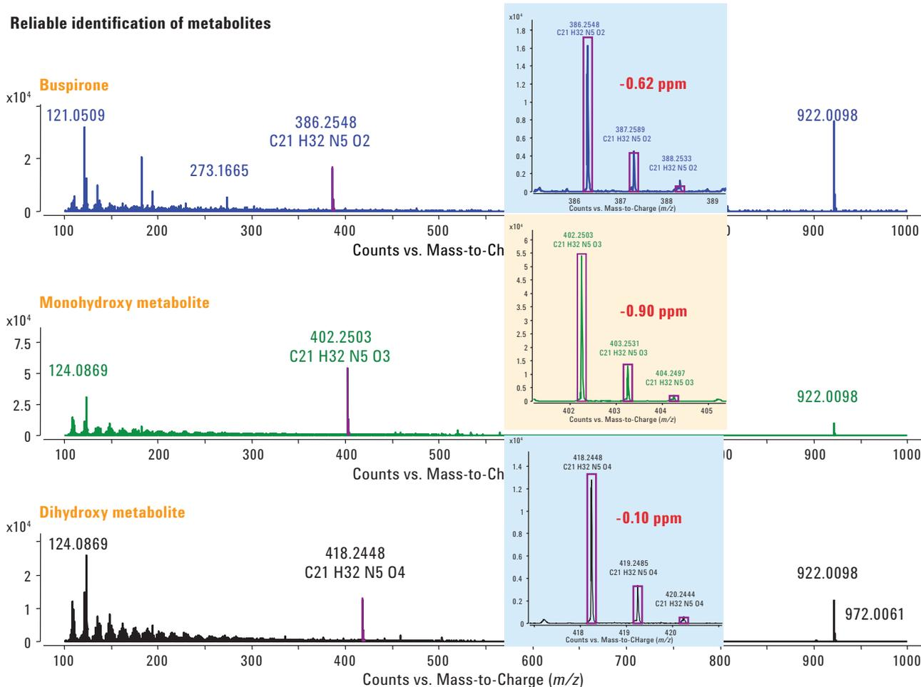
Figure 3. Metabolite spectra taken with the 6540 QTOF demonstrated excellent mass accuracy and isotopic fidelity, which provided assurance of correct identifications.
