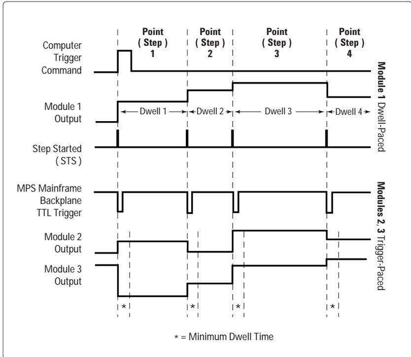
Figure 5. Timing Diagram for the Generalized Synchronizing Scheme
