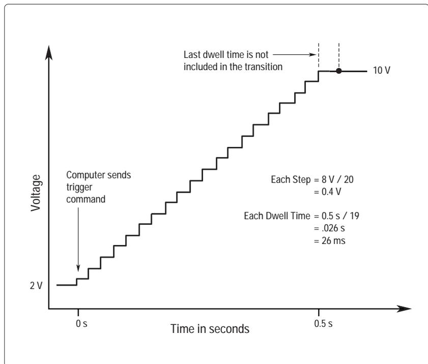
Figure 3-3. Generating the Desired Voltage Ramp for Application #3
