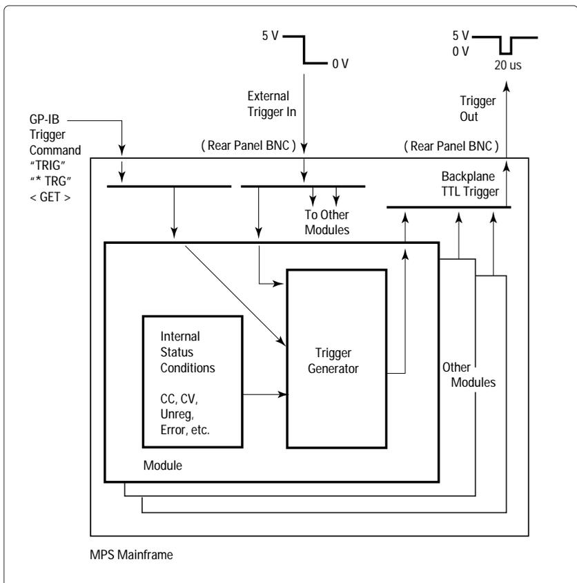
Figure 2. Generating TTL Triggers
