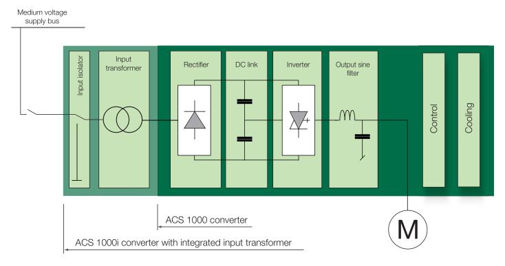
The ACS 1000 drives family's well proven three-level inverter, without series or parallel connected power semiconductors, is one of the least complex, most robust and efficient drive topologies.
