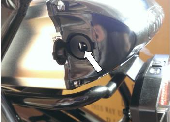
To charge the battery, simply lift the weatherproof cover and connect the charger to the socket and then plug the other end into a regular mains socket. On the charger is a small light which is red while charging. When charging is complete, this light will turn green.
