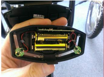
The front light may also have a insulating tag that needs to be pulled/removed. The front light uses 2x AA batteries. The on/off button is located on the top of the lamp. To change the batteries, press down on the small black clip at the base of the lamp, and lift the lamp/reflector clear. The batteries should be oriented as shown below.
