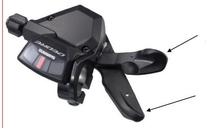
Pull with trigger finger to shift to the lower gears.
