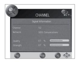
Position and align the antenna so that the maximum possible values for "Quality" and "Strength" are obtained.
