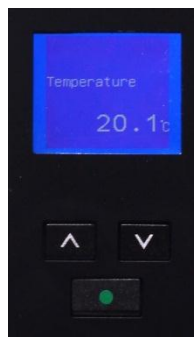
A dual-color LCD provides critical information and notification of alarm conditions
